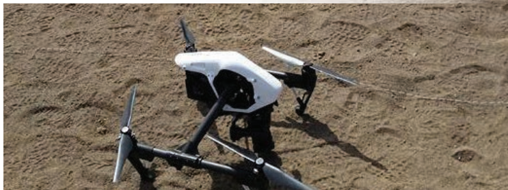
Multi-rotor UAV used to monitor eruption at Stromboli volcano. Stromboli is one of the Aeolian Islands off the coast of Sicily
