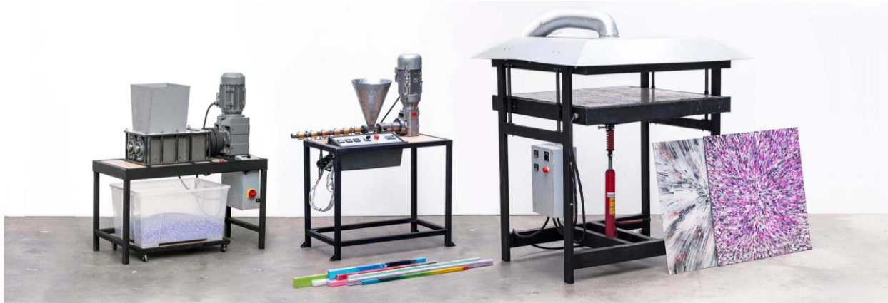
Figure 5: Precious Plastic semi-industrial open-source design recycling machines support decentralized waste management, Precious Plastic
